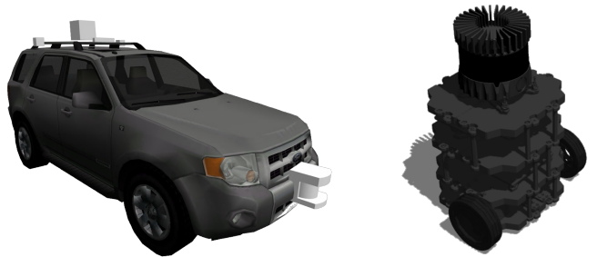
(a) Modified Catvehicle [30] simulation with 360° 64 layer Velodyne LiDAR: Ackerman steering
